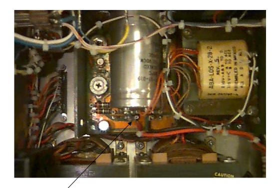
Measure this point to chassis. If working properly it will be 28 to 29V DC with less than 100mV AC ripple.
