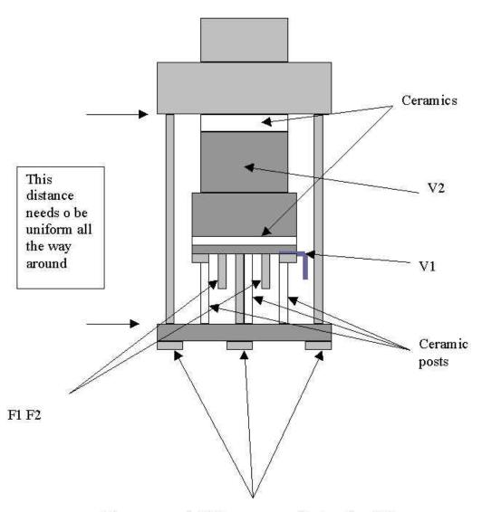
These screws hold the gun assembly together. It is stacked on the ceramics. Tighten it up, but not too much. All 3 screws should have the same distance with-in .001".
