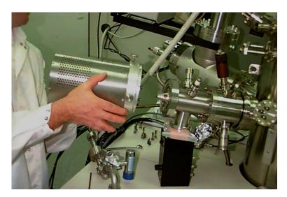
7. Prepare a work area and cover it with clean aluminum foil. Place the source on the work area and remove the outer shield. Remove the top heat sink.
