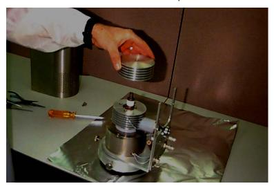
8. Remove the second heat sink (3 screws) and the 6 screws, which fasten the cathode ceramic to the source housing.
