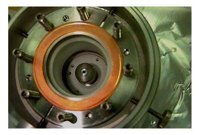
12. Remove the ceramic at the base of the source. Use a long needle nosed pliers, being very careful not to drop the ceramic.
