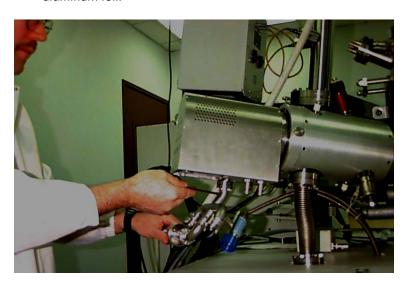
2. Disconnect the differential pumping line. Protect the knife-edge with aluminum foil.
