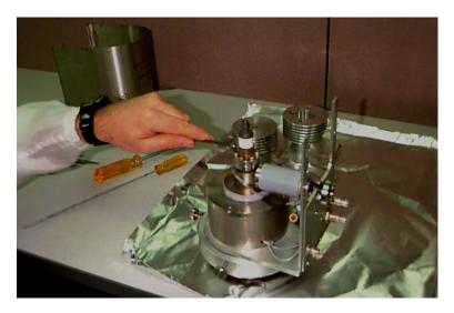
9. Remove the cathode ceramic by lifting it straight up. Tip: make a lip on the edge of the aluminum foil to capture the red sapphire beams which will fall out when the cathode ceramic is removed. These sapphire beads insulate the cathode from the intermeditate electrode (You can clean the nickel off of these beads with a small amount of diluted nitric acid and re-use them if you have access to a chemistry lab).
