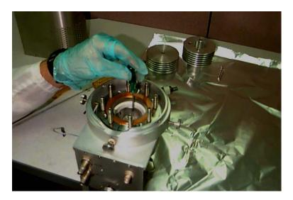
10. Turn the source over and remove the 4 screws, which hold the anode to the anode support housing. Use pliers to lift the anode out.
