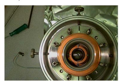
11. Remove the 4 screws (also the washers and ceramics) that hold anode support to the base of the source. Use a needle nosed pliers to lift the screws and washers out.
