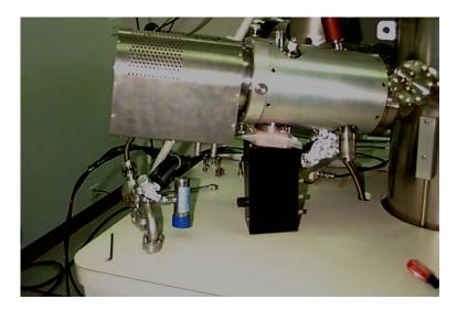
4. Remove the alignment collars by first removing the screws which hold the collar to the ion gun column. Be very careful when pulling the halves of the collar away from the COND and OBJ high voltage feedthrus.
