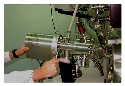
6. Carefully remove the source from the column.
