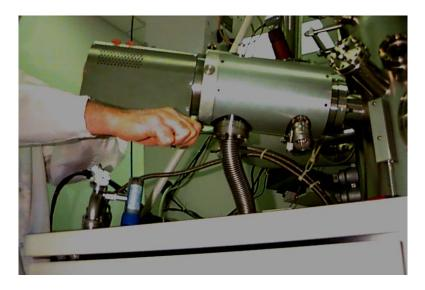
3. Support the differential pumping port with some solid object. Use aluminum foil to protect the knife-edge from becoming damaged. The reason that this needs to be supported is so that when the alignment collars are removed from the column the bellows plate will not be supporting the total weight of the ion gun. If this happens, the bellows plate may develop a vacuum leak.
