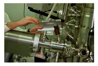
5. Remove the 8  $\frac{1}{2}$ " hex nuts, which fasten the source to the column. Be careful to support the source when you remove the last nut.
