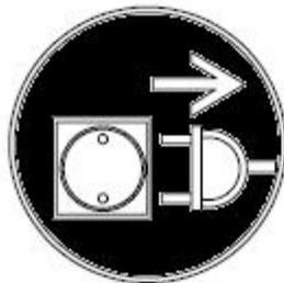
This symbol indicates that the equipment must be unplugged from its power source before any service or maintenance is performed on the equipment.
