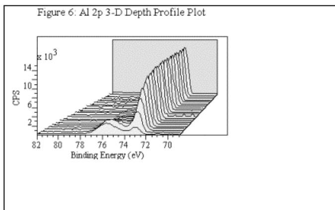
Figure 6 shows a plot of the Al 2p energy-region profiled against etch time. The data envelopes change in shape as the surface oxide layer is removed by the etch cycles to reveal the homogeneous bulk aluminium metal.
