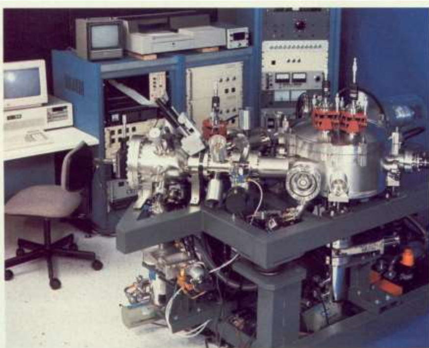
This direct imaging TOF-SIMS instrument offers high mass resolution, high lateral resolution, and rapid image acquisition in the ion microscope mode.
