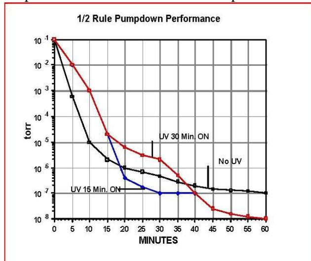
*Pumpdown performance is a function of the UV power/surface performance is a function of the UV power/surface area ratio and total UV exposure time. UV, properly applied, can provide either a faster pumpdown or a lower ultimate pressure.*
