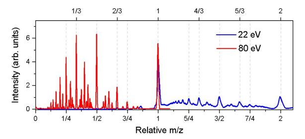
In the upper graph two measurements recorded at different electron energies with the Snowball experiment are displayed, which show that, contrary to what was accepted by the scientific community for many years, helium nanodroplets can hold a bevy of charges. This property makes them an ideal matrix for the production of ionic clusters for mass spectrometry and high yields of various nanoparticles which can be deposited on surfaces.
