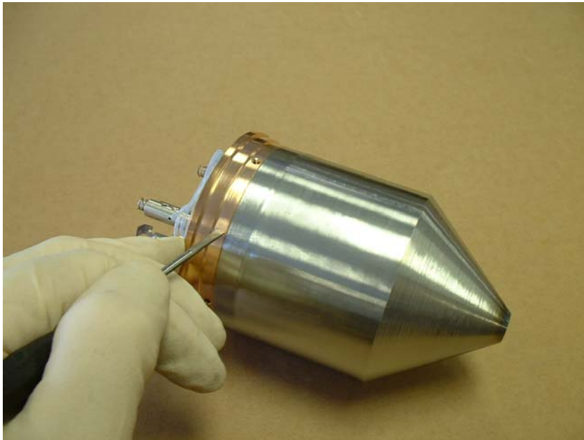
Figure 5. Scribe the objective assembly so that the nose cap may be realigned during reassembly.
