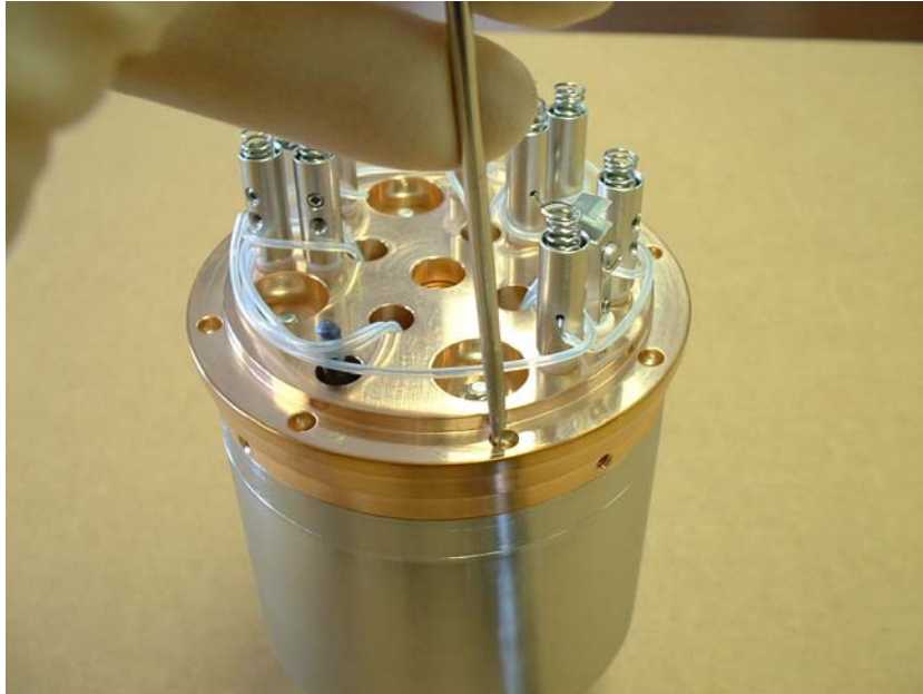
Figure 6. Removing the 8 screws which hold the nose cap in place.
