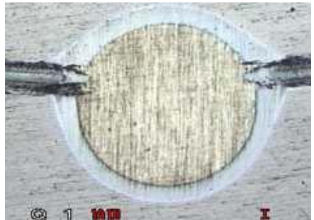
Figure 3 : Calotest crater made over a pin-on-disk tribometer wear track (test conditions; 5 N load, 10 cms-1 speed, 1 hour, ball diameter = 25.4 mm). Sample is TiAlN deposited onto a 100Cr6 substrate
