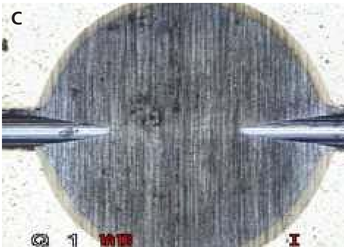
Figure 4 : Calotest craters produced on a RVT scratch track made on a TiN-coated steel sample (test conditions; 0-100 N progressive loading, 10 mm/min. speed, 200 m tip radius). The critical load (46.7 N) occurred in the central area of the crater. Micrograph (b) is a zoomed image of the left hand portion of (a), whereas (c) shows a deeper crater to below the scratch track.
