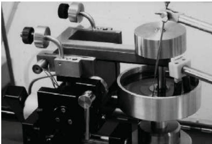
Figure 1 : Detail of the modified Tribometer with external heating element and thermocouple. The sample is completely submerged in the oil bath.
